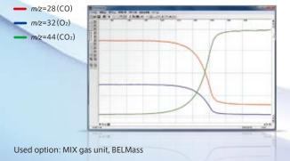
■ Temperature-programmed reduction (TPR) of supported palladium catalyst from low temperature (-100°C)
