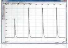
Adsorption amount: 0.566cm<sup>3</sup>/g Metal surface area: 1.22m<sup>2</sup>/g Metal dispersion degree: 25.4% Metal particle size: 4.7nm
