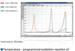
carbon monoxide using precious metal catalyst
